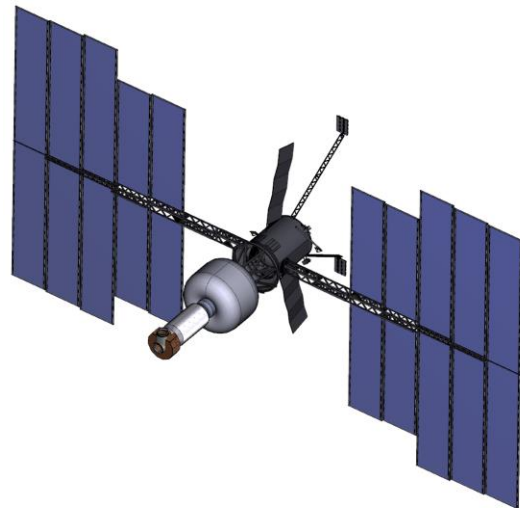
Figure 6. NASA Mars Transit Vehicle concept utilizing a Sierra Nevada inflatable habitat module.
