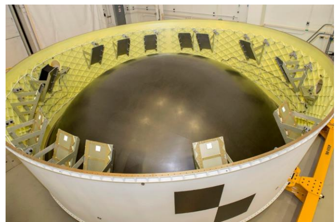
Figure 9. The completed Artemis I Orion Stage Adapter (OSA), which has volume for CubeSat payloads; brackets that hold the COTS dispensers are visible
