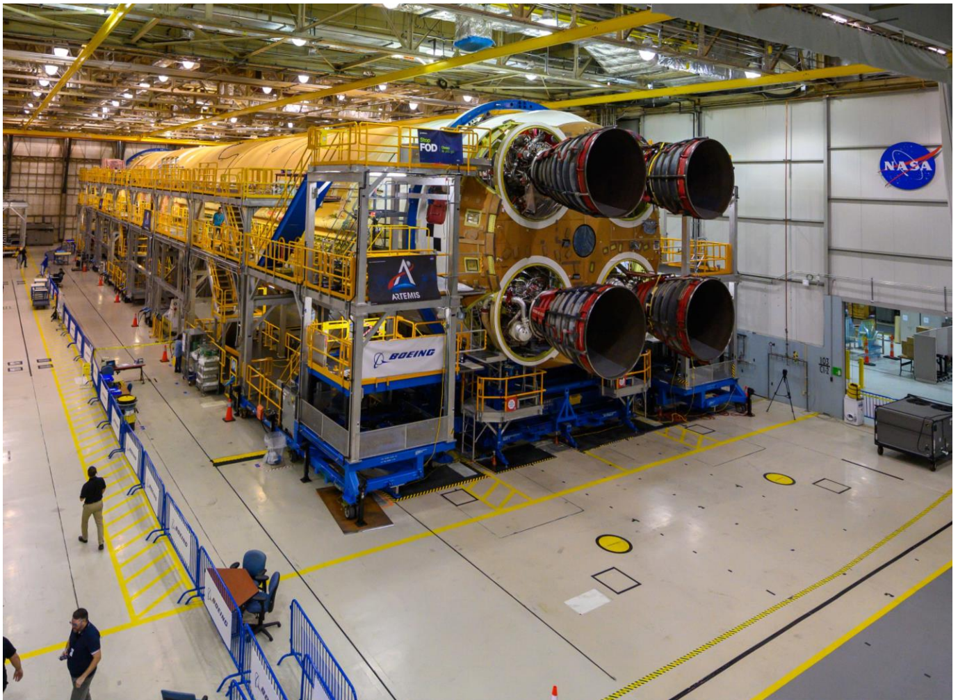
Figure 5. The SLS Program's major new development, the core stage, was completed in late 2019 and will ship to SSC for Green Run testing in 2020.
