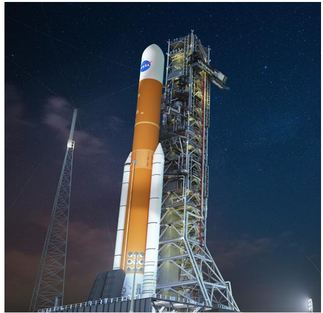
Figure 1. Artist's rendering of the Space Launch System (SLS) Block 1B with an 8.4 m-diameter fairing on the Mobile Launcher (ML) at Launch Complex 39B at NASA's Kennedy Space Center (KSC)
