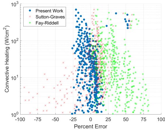
Figure 5: Comparison of convective heating predictions.
