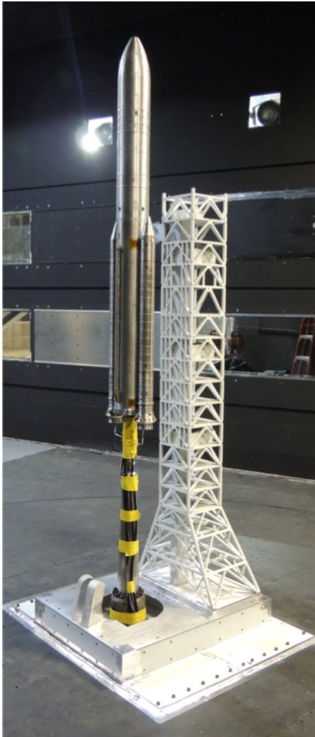
Fig. 3 SLS Block 1B Cargo (27005) configuration wind tunnel test article shown with the launch tower model in the 14x22 Wind Tunnel.
