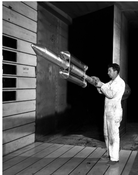
Fig. 6 A model of the Titan III in the Ames 14ft wind tunnel. Photo credit: NASA (ARC-1962-A-29073).
