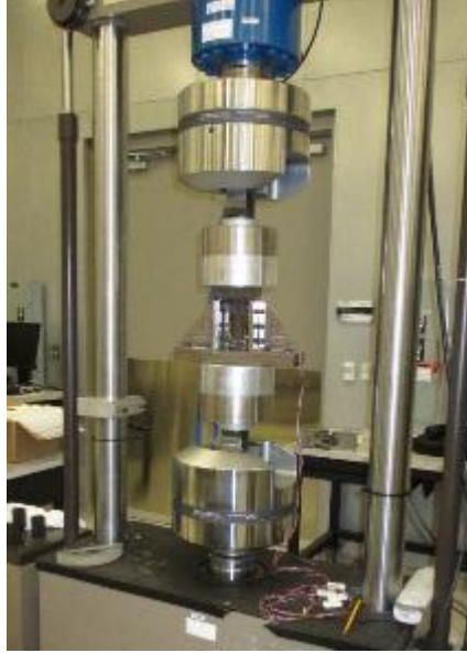
Fig. 7 CAI test specimen in hydraulic test frame.
