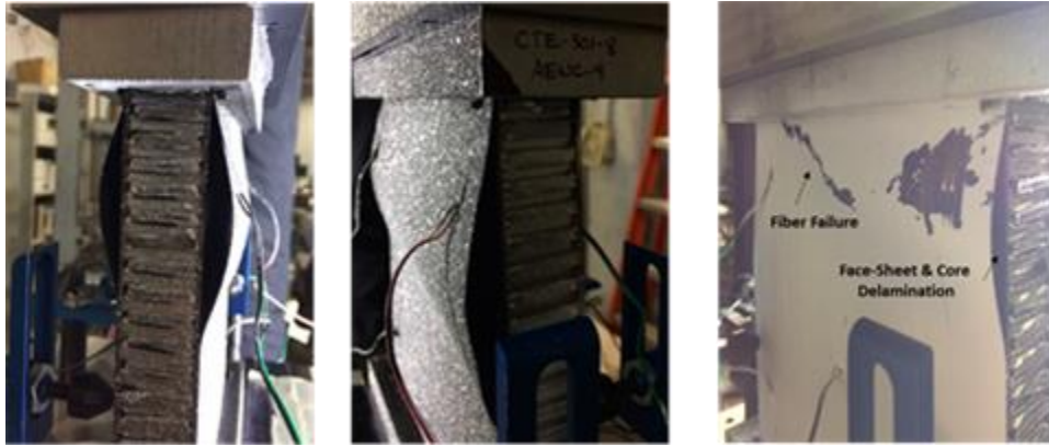
Figure 26 Failure Modes of Impacted AEW C Coupons.
