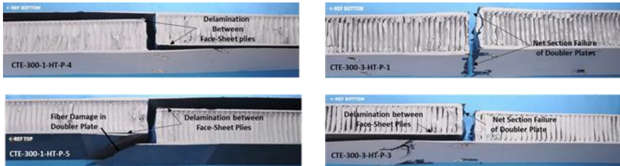
Figure 31 Typical Damage Modes in HEWT coupons.
