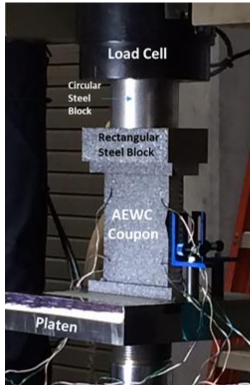
Figure 23 Test Setup & Strain Gauge Configuration of AEWc Coupon.
