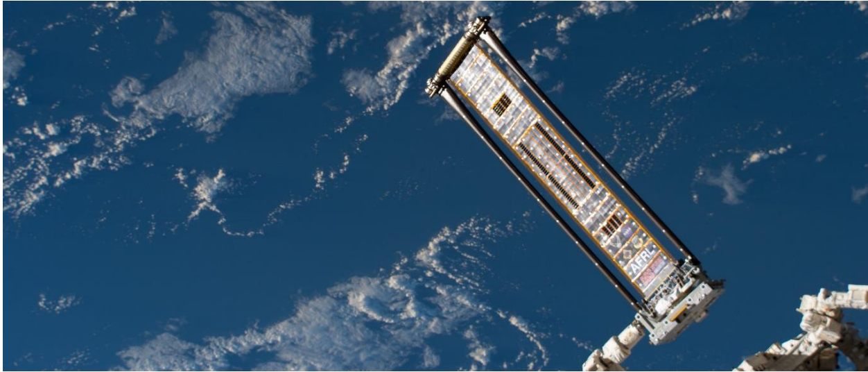
Fig. 1 ROSA flight experiment on ISS (note SPDM holding ROSA FRAM at bottom right)
