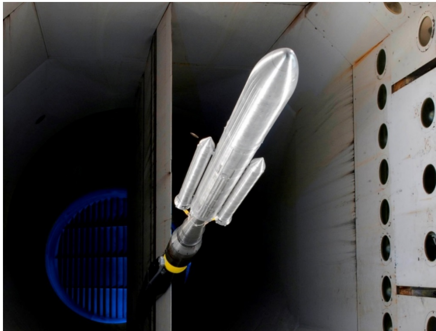
Figure 3. Space Launch System Block 1B cargo vehicle configuration in the Langley Research Center Transonic Dynamics Tunnel during 2012 wind-tunnel test program.
