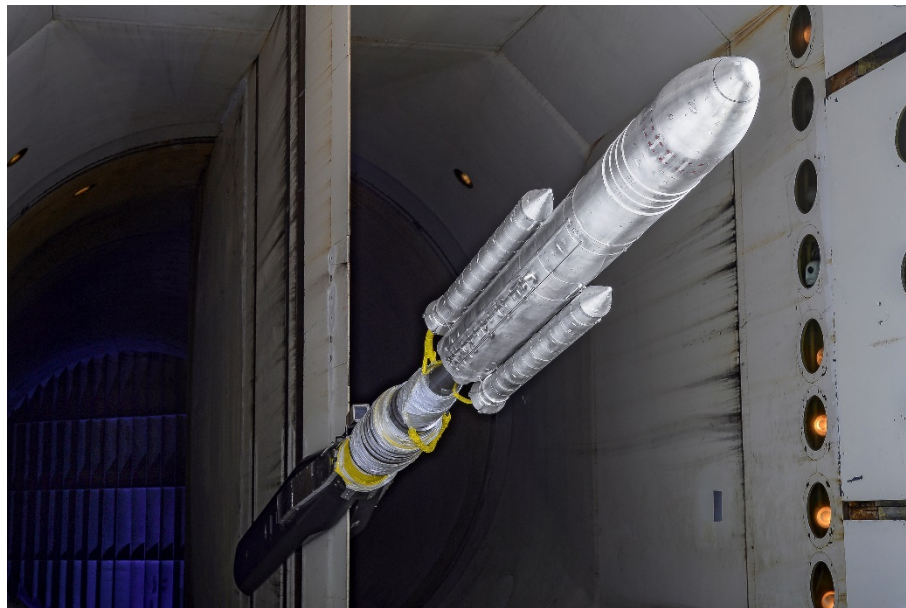
Figure 5. Space Launch System Block 1B cargo vehicle configuration with terminal shock arrays in the Langley Research Center Transonic Dynamics Tunnel during 2016 wind-tunnel test program.
