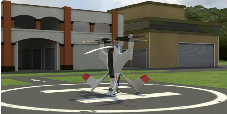
Fig. 3 NASA Puffin aircraft concept with stacked prop-rotors.
