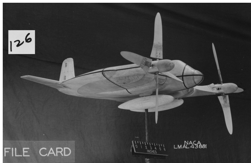
Fig. 2 XF5U-1 model from 1945 for the NASA Langley 20-foot spin tunnel [4].
