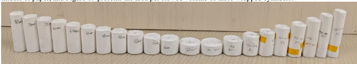
Figure 18: Entirely-parallel z-folded and cylindrically wrapped triangles of paper with different fold height and resulting wrapped diameters.
