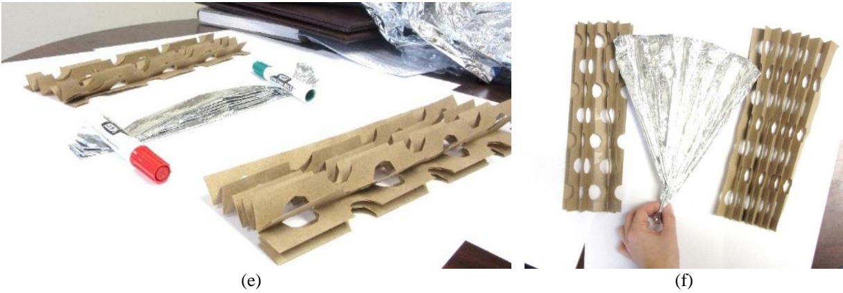
Figure 11: Removing the forms from the membrane. First (a), the membrane was pinched through an access hole in the paper folding form, shown in detail in (b). The paper folding form could be removed from one side (c). This operation was repeated to remove the other form (d) while restraining the membrane. The membrane was then free from its folding forms (e) and could be deployed (f).
