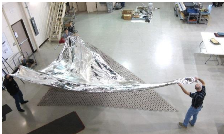
Figure 1: Folding a solar sail prototype triangular quadrant with a 9.2-meter edge for laboratory use.
