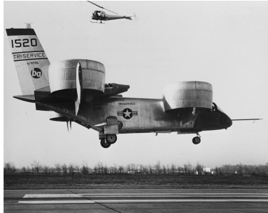
(a) Tilting duct: Bell X-22.[50]
