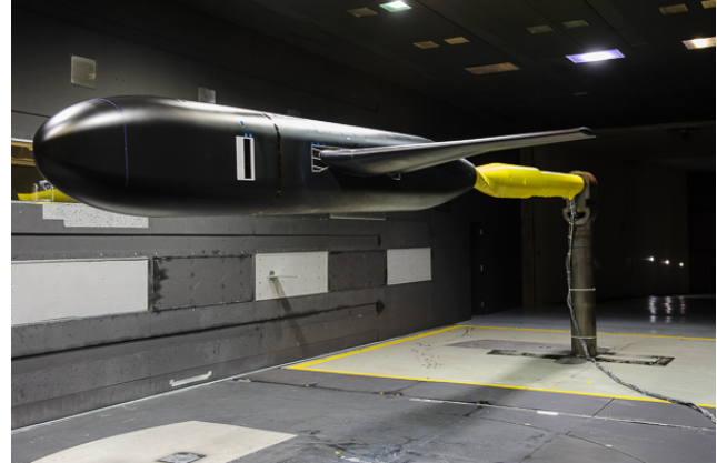
Figure 1: Junction model installed in the NASA Langley 14-by-22-Foot Subsonic Tunnel.
