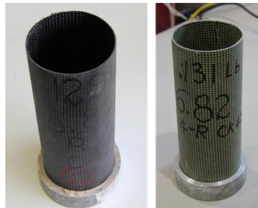
Figure 2 - Composite tube specimens. Traditional C/C (left), and C/A hybrid (right)
