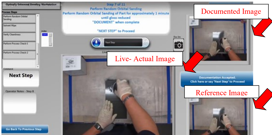
Figure 12. Bond Optimization Workstation - Sanding Process Step
