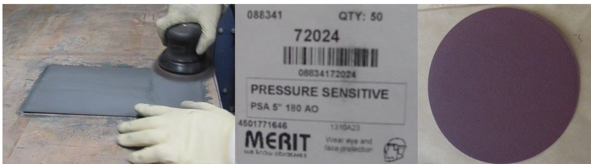
Figure 1. Manual ROS sanding process and materials for surface preparation of epoxy composite panels
