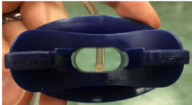
Figure 2. Mouth guard with sample probe inserted to perform sampling.
