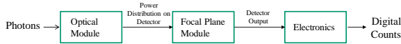
Fig. 1. Flow of signal chain for an instrument. Photons converted to digital counts.
