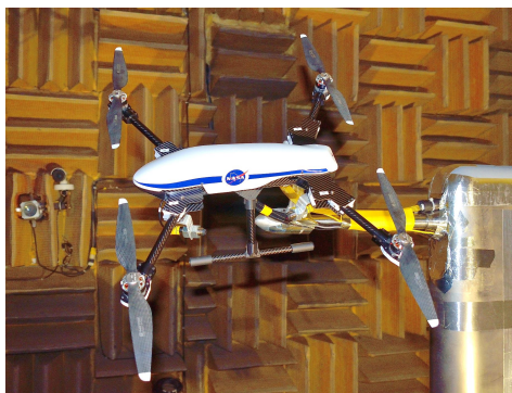
(a) Image of vehicle installed on MTS
