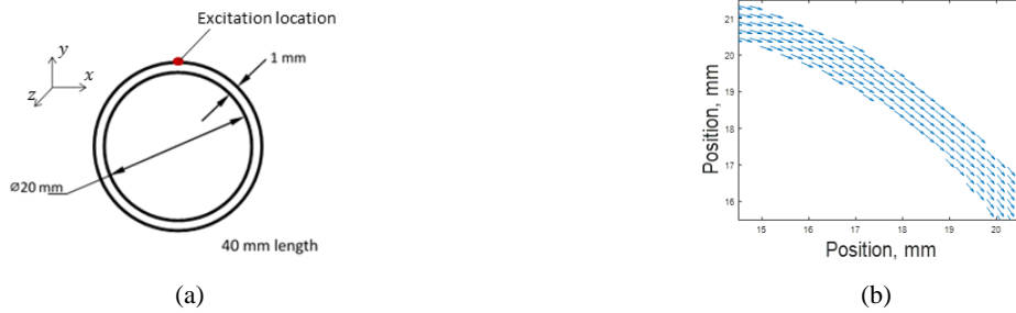
FIGURE 6. (a) Dimensions of a cylinder verification model, with (b) fiber oriented circumferentially around the cylinder
