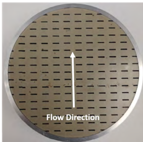
(a) Facesheet sample illustrating perpendicular flow slots.
