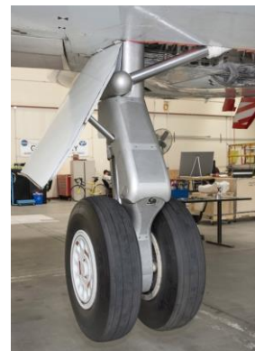
b) Fairings installed
