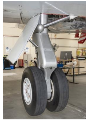
b) With fairings installed
