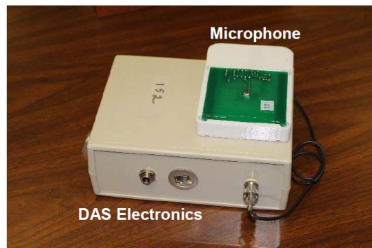
Figure 6. Microphone mounted on top of NeAR module.
