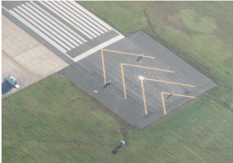
Figure 1. 167-microphone array at NASA WFF in 2006. Dots on overrun area are microphone ground plates. Data acquisition cabinets are visible around the array perimeter.
