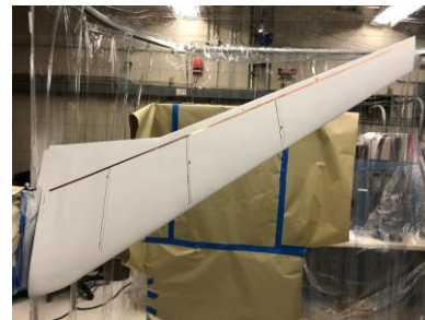
Fig. 4. Copper tape electrode placed near trailing edge on the upper surface of the CRM-NLF.
