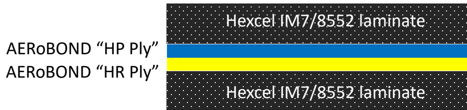
Figure 8. Configuration of AERoBOND laminates for mechanical testing.
