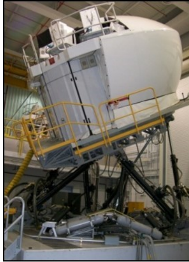
Fig. 2 A photograph showing the exterior of the simulator cockpit mounted on a hexapod motion base.
