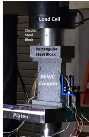
Figure 6. Test Setup & Strain Gauge Configuration of AEWC Coupon.
