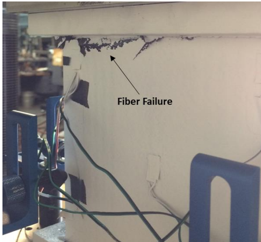
(a) Typical Failure Mode of AEW Coupon
