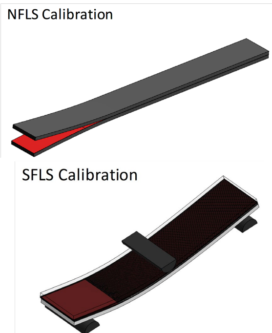
Figure 5 Calibration of tiebreak contact based on quasi-static fracture toughness test results
