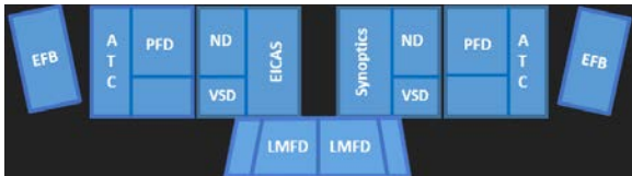
Fig. 5. AIME flight deck display layout.
