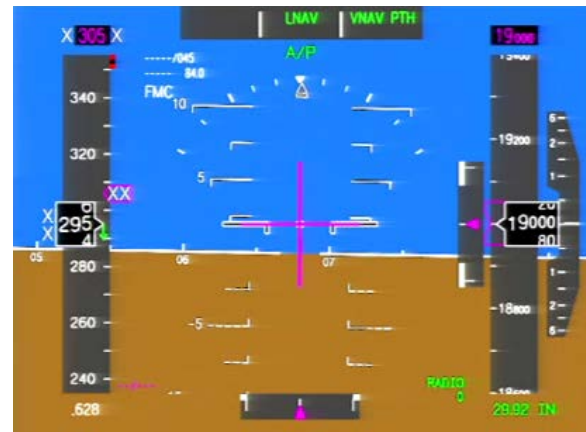
Fig. 2. EACI display at 10 kt airspeed loss after autothrottle failure. White XX’s indicate automation is not controlling to target airspeed.
