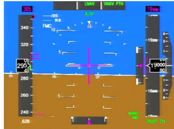
Fig. 1. BL display at 10 kt airspeed loss after autothrottle failure.
