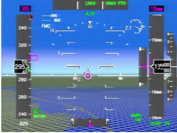
Fig. 3. FPV display at 10 kt airspeed loss after autothrottle failure. Note acceleration caret and speed deviation box below left wing of FPV symbol.
