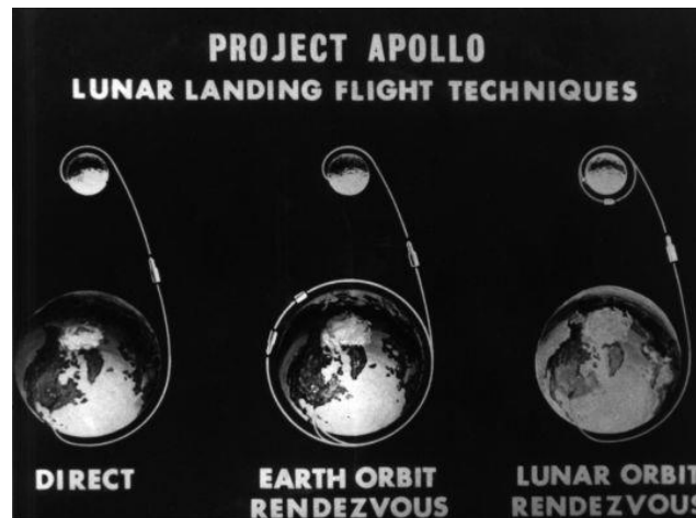
Figure 7. Three principal lunar landing techniques which were proposed for the Apollo program.
