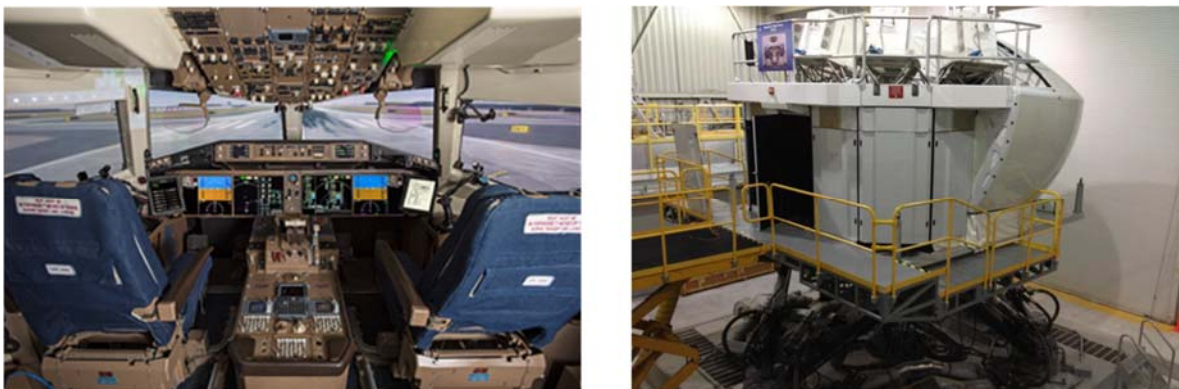
Fig. 8. RFD simulator interior (left) and exterior (right).
