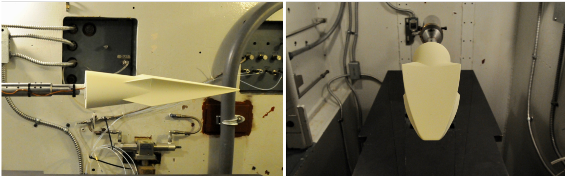
Fig. 3 Subscale BOLT model shown in the 20-Inch Mach 6 Air Tunnel in the retracted position.
