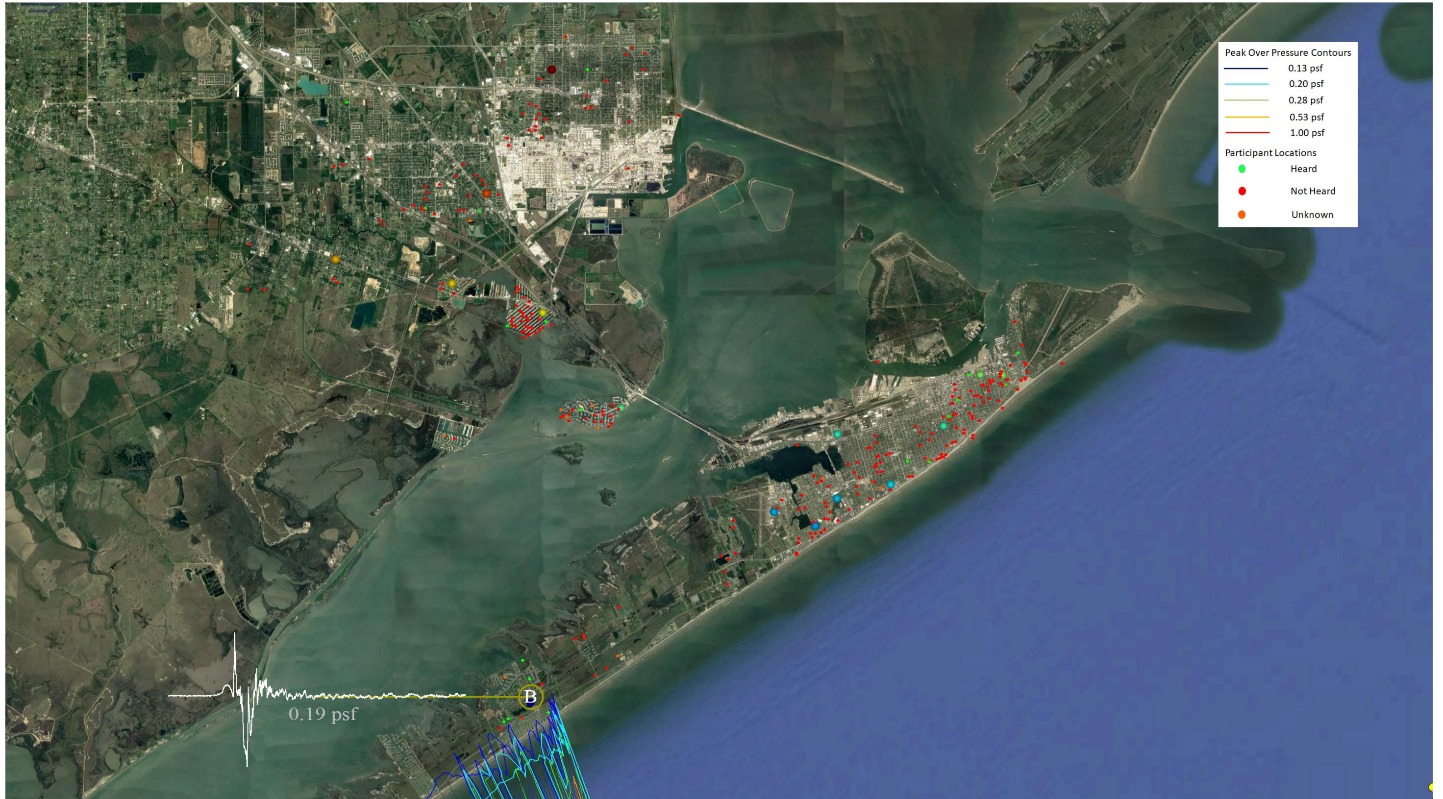
Figure 6-6 Calculated footprint showing peak overpressure contours from QSF001 with recordings and participant locations
