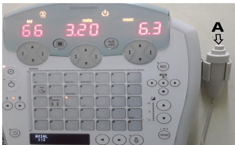
Figure 3.5: Control panel comprising of control buttons and exposure button (A)
