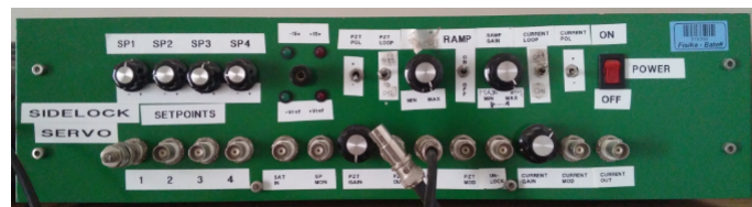
Figure 2.9: PID controller box
