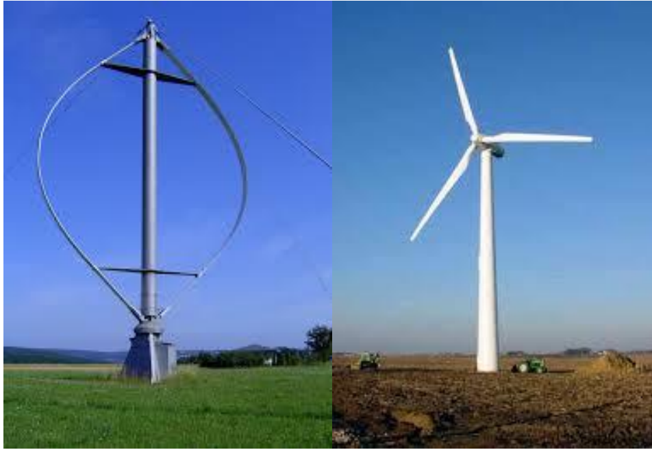
Figure 2.5: Wind turbine rotor configurations
