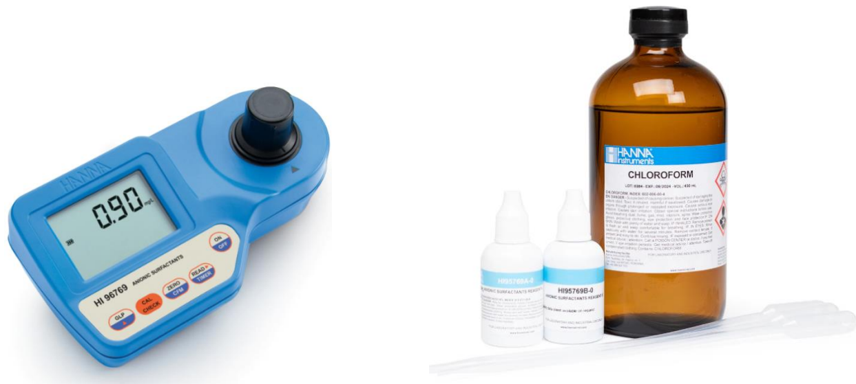
Figure 3-7: Anionic Surfactant Portable Photometer (left) and reagents (right)
