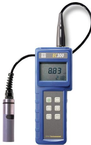
Figure 3-6: YSI Eco Sense EC300 conductivity meter model use during the experiments
