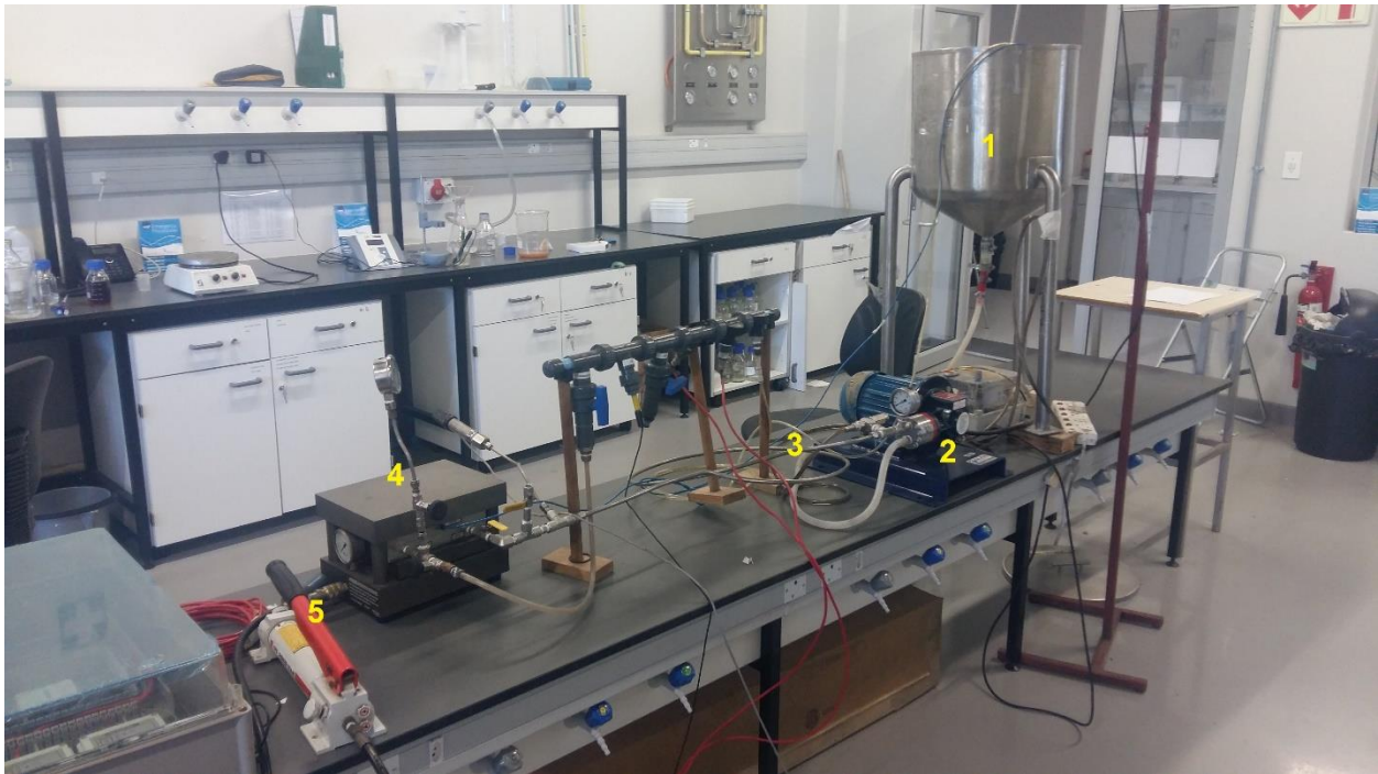
Photo 3-1: RO bench-scale unit in the Environmental Engineering water system laboratory (October 2019)
