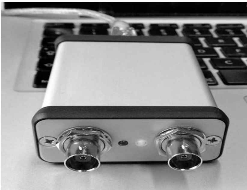
Figure 51: Low jitter precision GPSDO reference oscillator (2 Ports) (adapted from Riley, 2016)
