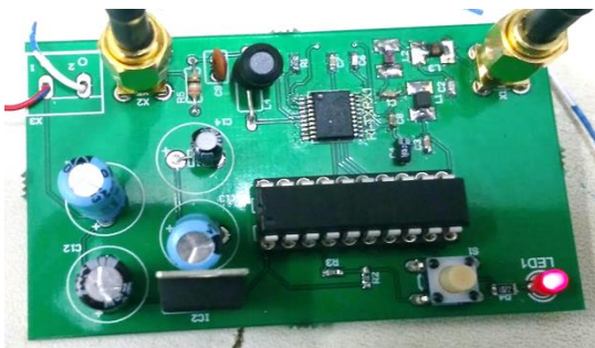
Figure 66: Morse controller section on a printed circuit board
