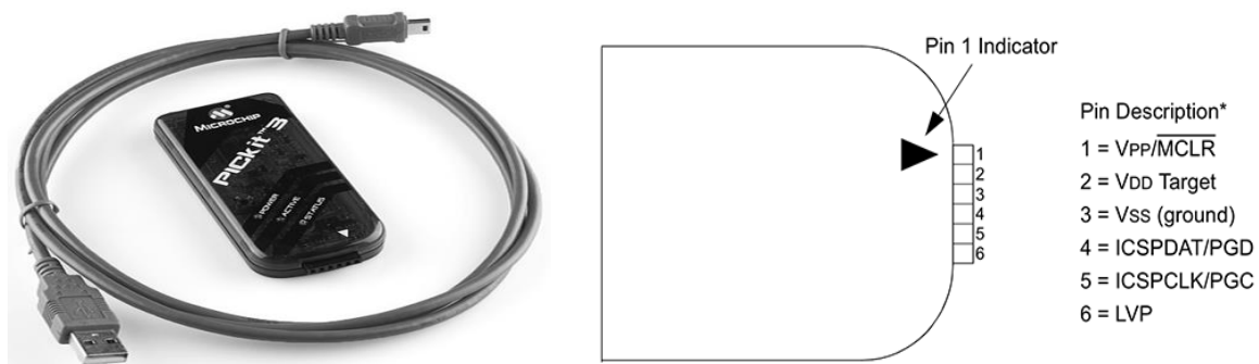
Figure 62: PICkit 3 and pin-out
