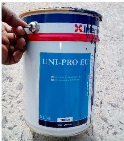
AF paint used on vessels at KB
