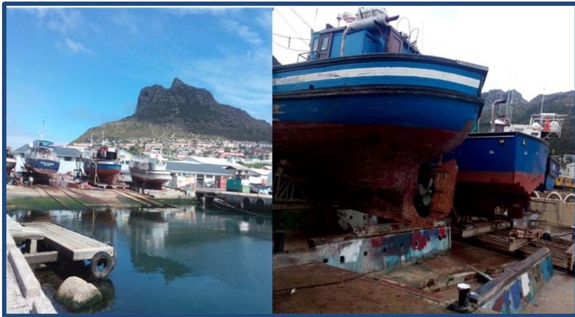
Figure 2. 4: Maintenance and repair of fishing vessels at a vessel repair facility adjacent to a slipway in Hout Bay Harbour (antifouling paint residue may enter near shore waters through runoff or wash down) (Source: Fru. W)
