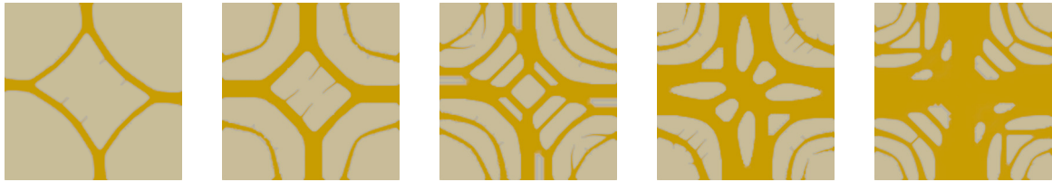
Figure 1.4: Optimal material distributions on a thin plate under certain volume conditions (here for different volume constraints). The hard material is colored in orange.
