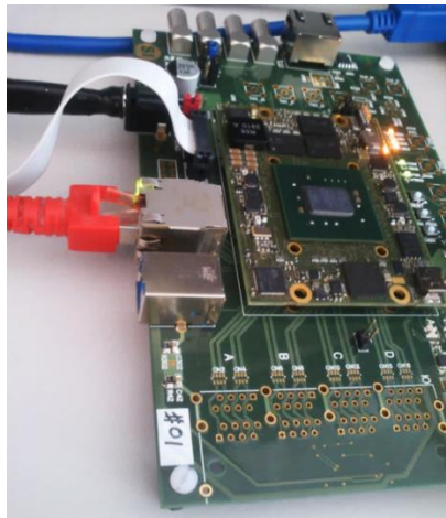
Figure 4.17: The MMC3 prototype board during the Ethernet test
