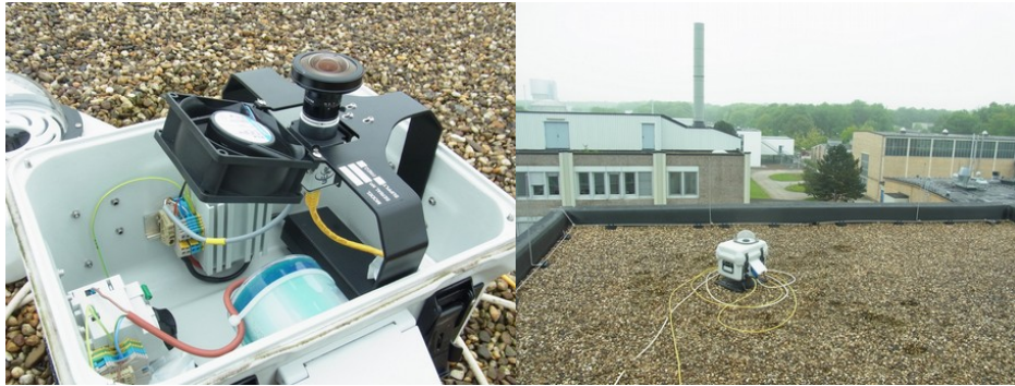
Figure 2.2: Left: Internal design of the hemispheric sky imager used in this study, including attached fan, metal mounting for the camera device, radiator and electric supply. Right: Sky imager on a roof within the Forschungszentrum Jülich GmbH.
