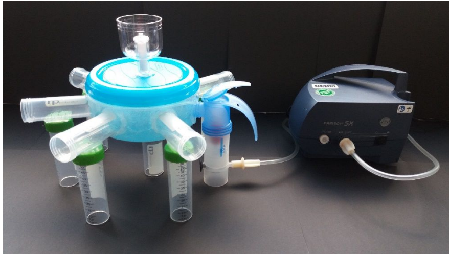
Fig. 2.3 Inhalation chamber to expose mice to aerosols. The home-made inhalation chamber is connected to a nebulizer system (Pari Boy SX, Pari).
