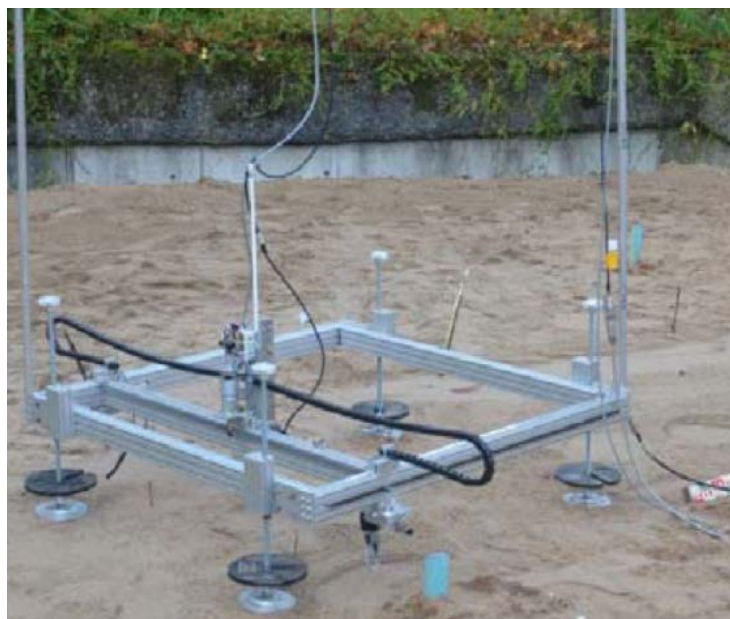
Figure 3.2: 3D laser scanner developed and custom-built for recording animal tracks. The scanner covers an area of 800 x 800 mm.
