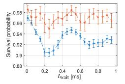
**Figure 5.9.** Losses in the compression procedure. Losses for the set containing initially 1 or 2 atoms (red squares) and initially containing more than 8 atom (blue circles) after a single compression sequence in a dipole trap at 860 nm and P = 112 mW with molasses cooling.
