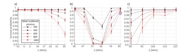
**Figure 4.5.** Survival probability for a given number of detected counts for different frequencies. Experimental data recorded using an illumination intensity of **a**)  $4I_{\text{sat}}$  and **b-c**)  $0.6I_{\text{sat}}$ , except for the last point in **c** ( $\Delta/2\pi = 123\text{MHz}$ ) where  $1.9I_{\text{sat}}$  was used. The blue circle for  $\Delta/2\pi = 85\text{MHz}$  corresponds to the example shown in Fig. 4.4. The lines are a guide to the eye.
