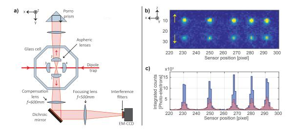
**Figure 2.13.** Single atom imaging. **a)** Sketch of the imaging optics. **b)** Image taken with the EMCCD camera. The upper row of atoms is the "normal" image, and the lower row is the image obtained using the reflected light. The reflected image is mirrored along the *x* axis as illustrated by the arrows. **c)** Integrated number of counts along the vertical direction for the normal and reflected images.
