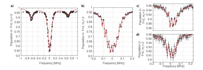
**Figure 5.5.** Raman Spectrum in a deep trap for <sup>87</sup>Rb. **a)** Full vibrational spectrum using a power of 36 mW for each arm  $(U_0 \approx 1.6 \, \text{mK})$ . The solid line is a fit to three equidistant Lorentzian curves **b)** Zoom into the carrier peak. The solid line is a fit to the radial sidebands using 15 equidistant Lorentzian curves. **c)** Same as **b** but for the heating (left) sideband. **d)** Same as **b** but for the cooling (right) sideband.
