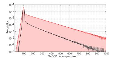
**Figure 2.15.** *Noise histograms*. Normalized histogram for the detected counts per pixel using the EMCCD camera for dark images (black lines and transparent area) and stray light from illumination (red lines and shaded area). The dark lines are fits to Eq. (2.21).
