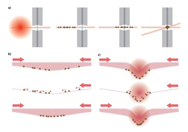
**Figure 6.2.** Creation of dense ensembles inside the resonator **a**) From left to right. Atoms are loaded in the MOT, transferred into the dipole trap, and transported inside the cavity using the optical conveyor belt technique. Then a compression sequence using the crossed traps is applied to increase the density of atoms inside the resonator. **b**) Compression scheme using a single standing wave. **c**) Second compression sequence using the crossed dipole traps.
