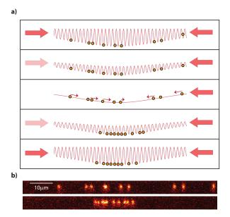
**Figure 5.7.** Atomic compression scheme. **a)** Schematic representation of the compression procedure. The wavelength has been scaled by a factor of 10 for better visualization of the standing wave potentials. In this method, one of the beams is adiabatically switched off for a small time and turned on when the density of atoms is maximum at the center. **b)** Image of atoms in the dipole trap before and after a compression sequence.
