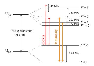
**Figure 2.6.** Relevant <sup>87</sup>Rb  $D_2$ -line levels. The cooling laser can be tuned to the  $F = 2 \rightarrow F' = 3$  transition. The other light frequencies are fixed at the indicated transitions (frequency splittings are not up to scale and Zeeman levels are not shown).
