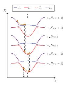
**Figure 3.4.** Photon scattering in the near-resonant field dressed-states picture. An atom is trapped in a dressed state potential and it jumps to another one by removing one photon from the near-resonant field and emitting it into free space.
