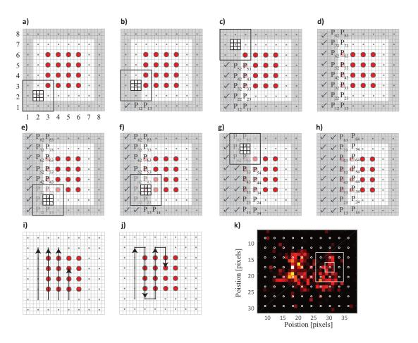
**Figure 4.14.** Bayes update scheme for a 2D lattice **a)-h)** Schematic diagrams showing the steps for the Bayesian update algorithm in a 2D image. The dark shaded regions represent the pixels from which the information has already been used, and the red circles represent the positions where atoms are located. **i,j)** Possible paths for the update algorithm. **k)** Sample of an image generated in the simulation.
