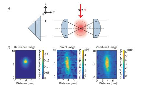
**Figure 2.14.** Collection efficiency. **a)** Dipole emission for  $\sigma$  light illumination. **b)** Stacking result for reference images (left), fluorescence collected with only one lens (middle), and fluorescence collected using also the Porro prism (right).
