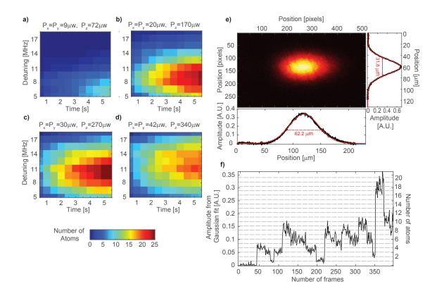
**Figure 2.8.** *MOT characteristics.* **a-d)** Number of atoms loaded in the MOT for different powers and frequencies. **e)** Image of the MOT acquired by the EMCCD. The plots at the right side and at the bottom show a Gaussian fit to the integrated image and the full width half maximum obtained from the fit. **f)** Variation of the fluorescence in the MOT as a function of time.
