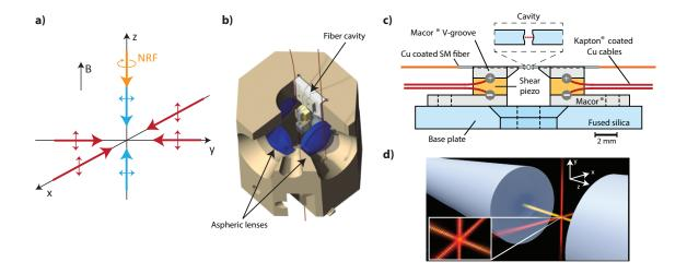
**Figure 6.1.** 3D optical lattice inside an optical cavity. **a)** Beam configuration for a 3D optical lattice that allows non-destructive state dependent fluorescence. **b)** Optical-fiber-based cavity combined with the lens system. **c)** Schematic representation of the actively stabilized fiber cavity. **d)** Artistic view of a 3D lattice created inside the resonator.
