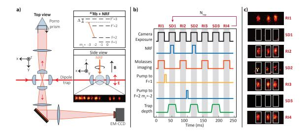
**Figure 4.3.** State detection sequence. **a)** Experimental setup and configuration of the near-resonant field (NRF). **b)** Simplified diagram of the sequence used to characterize the state detection. Reference images (RI) and state detection images (SD) are acquired alternately. **c)** Typical sequence of reference images and state detection images acquired with the EMCCD camera in one iteration of the experimental sequence.
