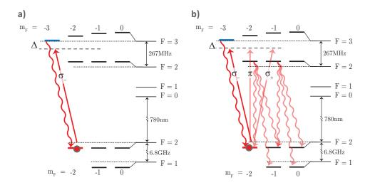
**Figure 4.1.** Cycling transition for <sup>87</sup>Rb. **a)** Ideal closed cycling transition for <sup>87</sup>Rb trapped in an optical dipole trap. Just the relevant hyperfine levels and part of the Zeeman spectrum are shown. **b)** Effect of polarization contamination on the closed transition
