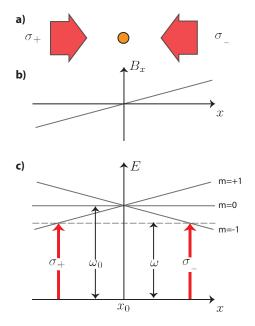
**Figure 2.5.** Working principle of a MOT **a**) Two counter-propagating beams, with a frequency  $\omega$  and opposite circular polarization interacting with a two-level neutral atom with a resonance frequency  $\omega_0$ . **b**) Position dependence of the MOT's magnetic field. **c**) Position dependence of the energy splitting for the Zeeman sub-levels.
