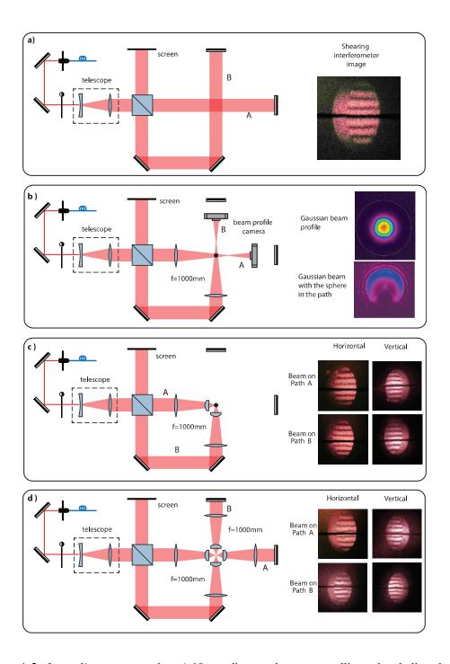
**Figure A.2.** Lens alignment procedure.**a)** 10 mm diameter beams are collimated and aligned with respect to the table. **b)** Compensation lenses are placed and the sphere is introduced by using the beam profile camera to measure its position. **c)** The aspheric lenses are aligned by monitoring the reflected signal in the screen and using the shear plate interferometer. **d)** The two last aspheric lenses are aligned.
