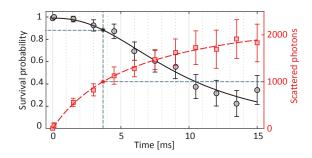
**Figure 4.4.** *Determination of survival probability for a given number of counts.* Measured survival probability (black circles) and mean number of scattered photons (red squares) for an atom in the bright state and  $\Delta_{\rm NR}/2\pi=85\,\rm MHz$ . The solid and long-dashed lines are the phenomenological fits. The short-dashed straight lines exemplify the determination of the survival probability for 1000 scattered photons.
