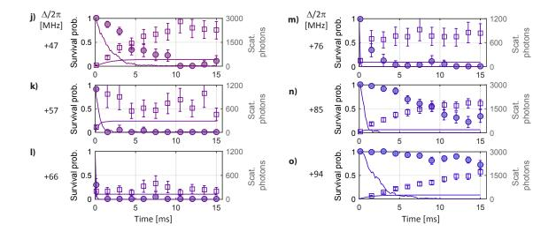
**Figure 3.6.** Photon scattering and atom survival for near-resonant illumination. **j-o**) Survival probability (circles), number of scattered photons (squares) and Monte Carlo simulation (solid lines) close to the AC-Stark shifted resonance at the bottom of the trap (~ 79 MHz) using the weak resonant illumination model (see Sec. 3.1.3). The error bars represent 95% confidence level. The same experimental data is shown in Fig.3.5 with the same indices.
