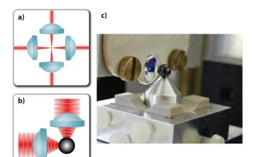
**Figure A.1.** Lens alignment using a highquality sphere. **a)** Desired lens configuration. **b)** The wavefront of a focused Gaussian beam matches the curvature of a sphere and is reflected. **c)**  $Si_3N_4$  sphere used for the alignment procedure.
