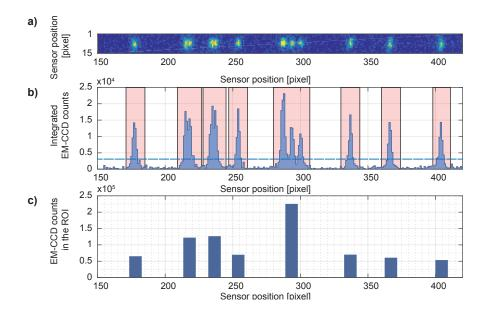
**Figure 2.16.** Determining the region of interest. **a)** Image acquired using the EMCCD with an exposure time of 20ms. The image also includes the reflected light using the Porro prism. **b)** Integrated profiles. The readout offset has been already subtracted. The horizontal dashed line is the initial threshold and the shaded areas represent the regions of interest. **c)** Total number of counts in each region of interest.
