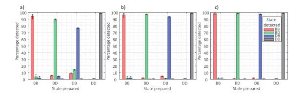
**Figure 4.10.** Bayes update result for atom pairs. Detection probability for every possible outcome for atom pairs prepared in different states, P(S'|S). **a-c**) corresponds to separations of 1, 2 and 3 lattice sites respectively. The error bars are obtained by bootstrap resampling.
