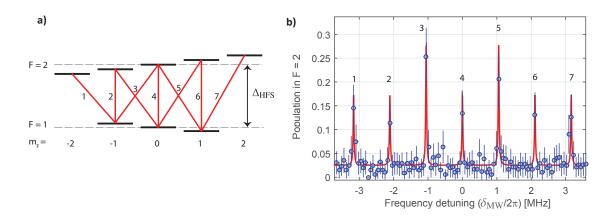
**Figure 5.1.** *Microwave spectroscopy of* <sup>87</sup>*Rb ground states.* **a)** Ground state levels and allowed MW transitions for <sup>87</sup>Rb. **b)** Experimental measurement of the MW spectrum. The red solid line is a fit of 7 equidistant Lorentzian curves to the experimental data.
