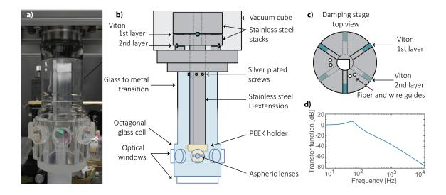
**Figure 2.3.** Glass cell and damping Stage. **a)** Octagonal glass cell mounted on the vacuum chamber with the set of aspheric lenses inside. **b)** Diagram showing the set of aspheric lenses mounted inside the chamber via the damping stage. **c)** Top view of the damping stage. **d)** Calculated transfer function for the two-stage vibration isolation system.
