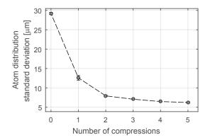
**Figure 5.12.** Distribution of atoms in the trap after different iterations of the compression sequence. The results are obtained for molasses-cooled atoms in a dipole trap at 860 nm with  $P = 112 \,\text{mW}$  and a free oscillation time  $t_{\text{wait}} = T/4$ .
