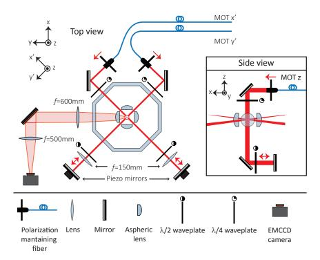
**Figure 2.7.** Simplified MOT setup. Light from the cooling  $(F = 2 \rightarrow F' = 2)$  and repumping  $(F = 1 \rightarrow F' = 1)$  transitions comes out of the optical fibers and it is retro-reflected creating the six cooling beams.
