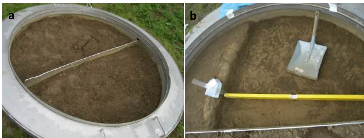
Figure 4.1: a) Metallic plate insertion in lysimeter top soil, b) Soil removal for digestate mixing.
