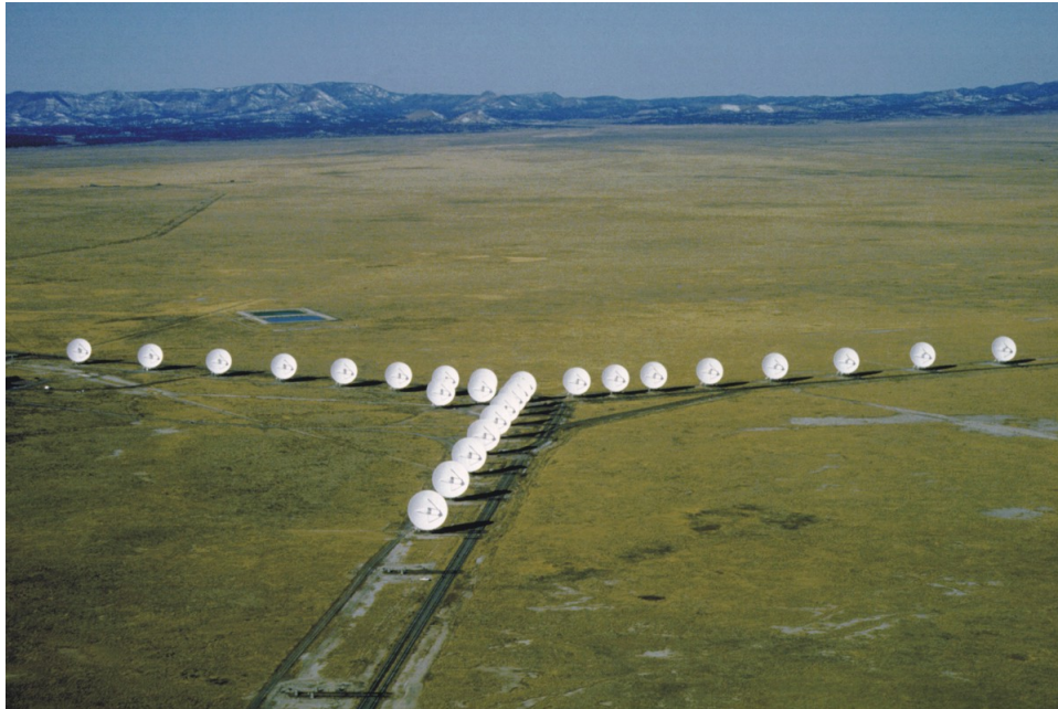
Figure 1.29: Aerial photo of the Very Large Array (VLA) in the high plains of San Augustin in New Mexico, USA, depicting its “Y”-shape in the most compact configuration. © NRAO, Associated Universities, Inc.
