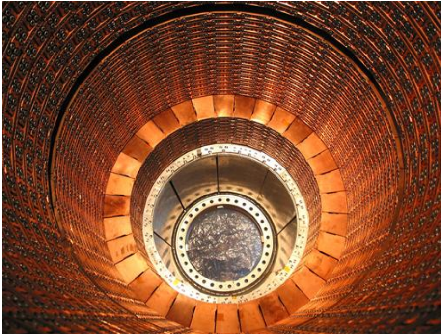
Figure 3.11: Picture of the inside of the ECAL [79].
