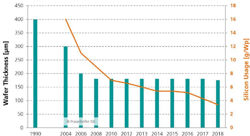
Figure 28. Changes in wafer thickness and silicon usage in c-Si
