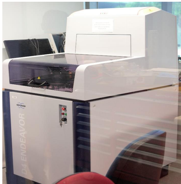
Figure 3.7: Cu K_{\alpha} ; Bruker D4 ENDEAVOR with Lynx-Eye PSD
