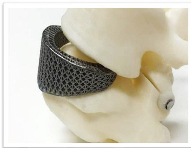
Figure 1. 1: 3D-printed titanium cage to fit perfectly into the spine[10].
