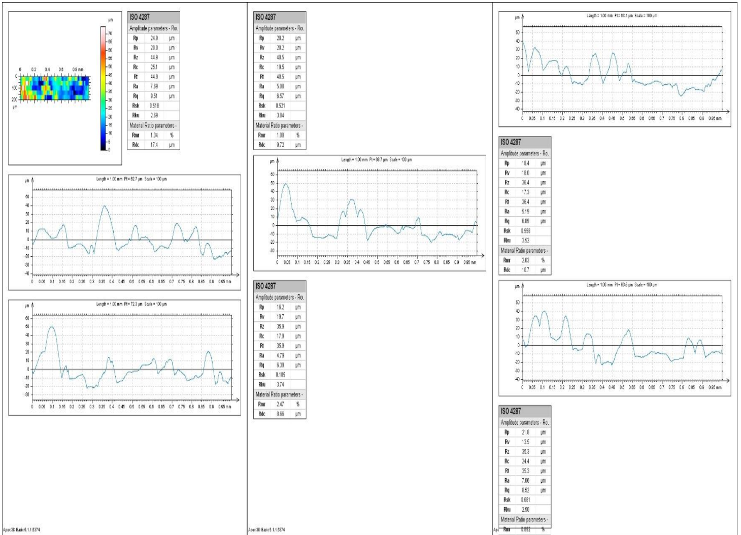
Figure 5.3.2: Surface profile properties for 45 degrees inclination such as maximum peak height ( R_p ), maximum valley depth ( R_v ), arithmetic average of roughness profile ( R_a ), root mean square deviation of the roughness profile ( R_q ), skewness of the roughness profile ( R_{sk} ), kurtosis of the roughness profile ( R_{ku} ) obtained by profilometer for 5 consecutive scans.
