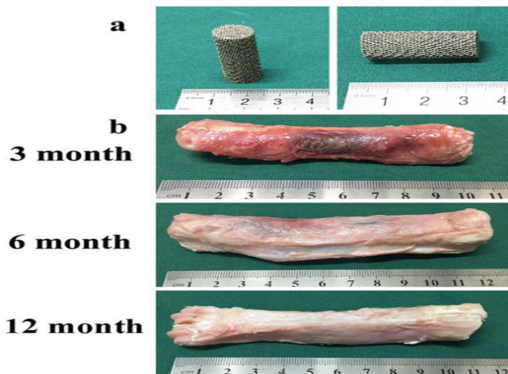
Figure 2.7: Additively manufactured Ti6Al4V scaffolds used for in-vivo experiment with a height and diameter of 30 and 10 mm (a) gross specimens at different time points (3 months, 6 months and 12 months) (b)[84].
