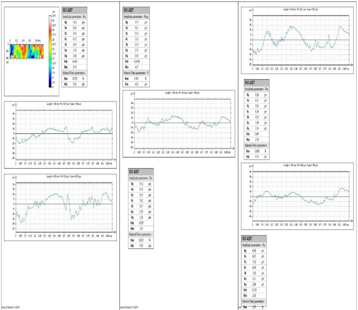
Figure 5.3.1: Surface profile properties for 0 degree inclination such as maximum peak height ( R_p ), maximum valley depth ( R_v ), arithmetic average of roughness profile ( R_a ), root mean square deviation of the roughness profile ( R_q ), skewness of the roughness profile ( R_{sk} ), kurtosis of the roughness profile ( R_{ku} ) obtained by profilometer for 5 consecutive scans
