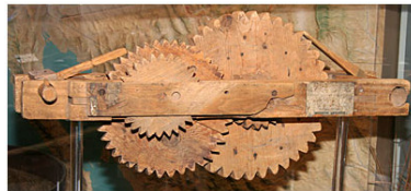
Figure 2.3: Roadometer, first used in May, 1847 [7].
