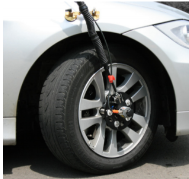
Figure 2.10: WPT sensors from Kistler Automotive [20].
