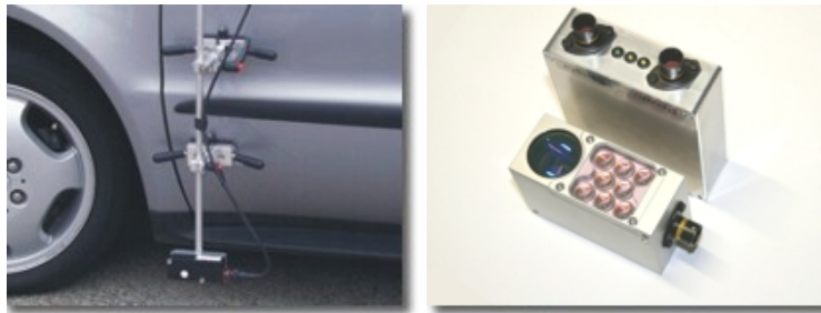
Figure 2.11: 2-Axis Non Contact Optical Velocity and Slip Angle Sensors [21].
