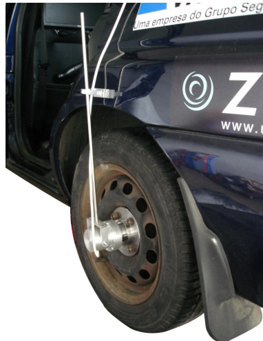
Figure 1.3: Velocity measurement system on ATLASCAR [3].
